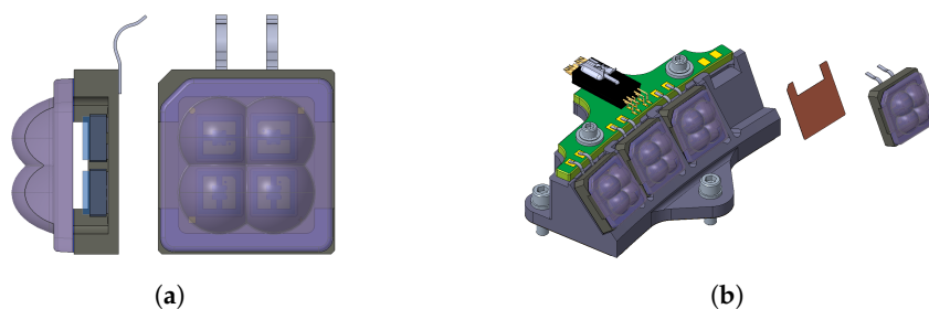
Figure 6. The fundamental, modular components comprising the UV rings. (a) A light engine consisting of a 2 \times 2 diode array and an aspheric microlens array. (b) A module consisting of 4 light engines, a PWB and a heat sink.
