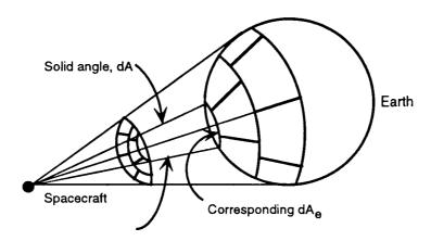
The incremental areas are found by dividing the solid angle subtended by the Earth from the spacecraft's point of view into NA solid angles of equal size (dA), each one corresponding to a piece of the Earth (dA $_{\rm e}$ ). Once the areas are defined, the necessary unit vectors are calculated for each area.
