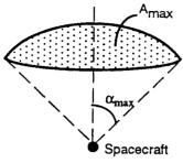
spherical segment with a half cone angle of  $\alpha_{max}$ , corresponding to the spacecraft's field of view. The surface area of this unit cone is equivalent to the solid angle subtended by the Earth,  $A_{max}$ .
