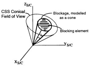
The first, second, and third elements are the components of a unit vector along the axis of the blockage cone in spacecraft body coordinates. The fourth element is  $\lambda$ , the half-angle of the blockage cone:
