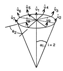
In addition to  $\hat{u}_1$ , define eight more unit vectors at an angle of  $\alpha_2$  from the axis of the field of view cone, equally spaced around the axis in increments of  $\theta_2$ , where  $\theta_2 = \frac{360^{\circ}}{8}$ .
