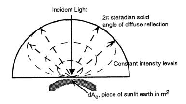
To determine the strength of the diffuse reflectance at the spacecraft's position, consider the geometry shown;
